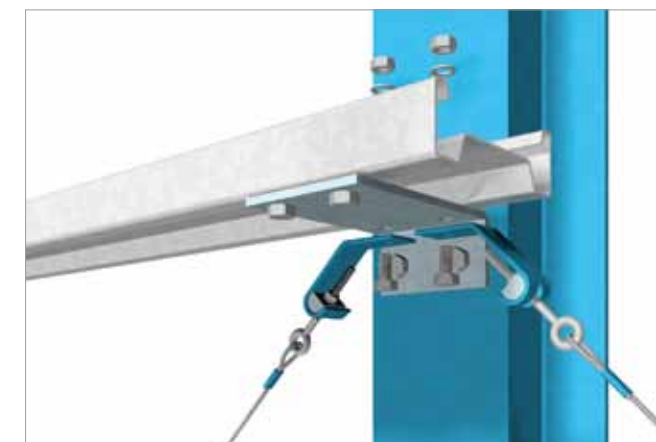
Construction detail of side rail + cleat + diagonal tie wire.
