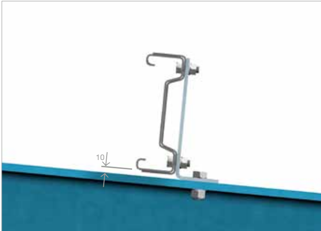
+/- 10 mm clearance between SadeF SIGMA-sections and substructure is recommended.
